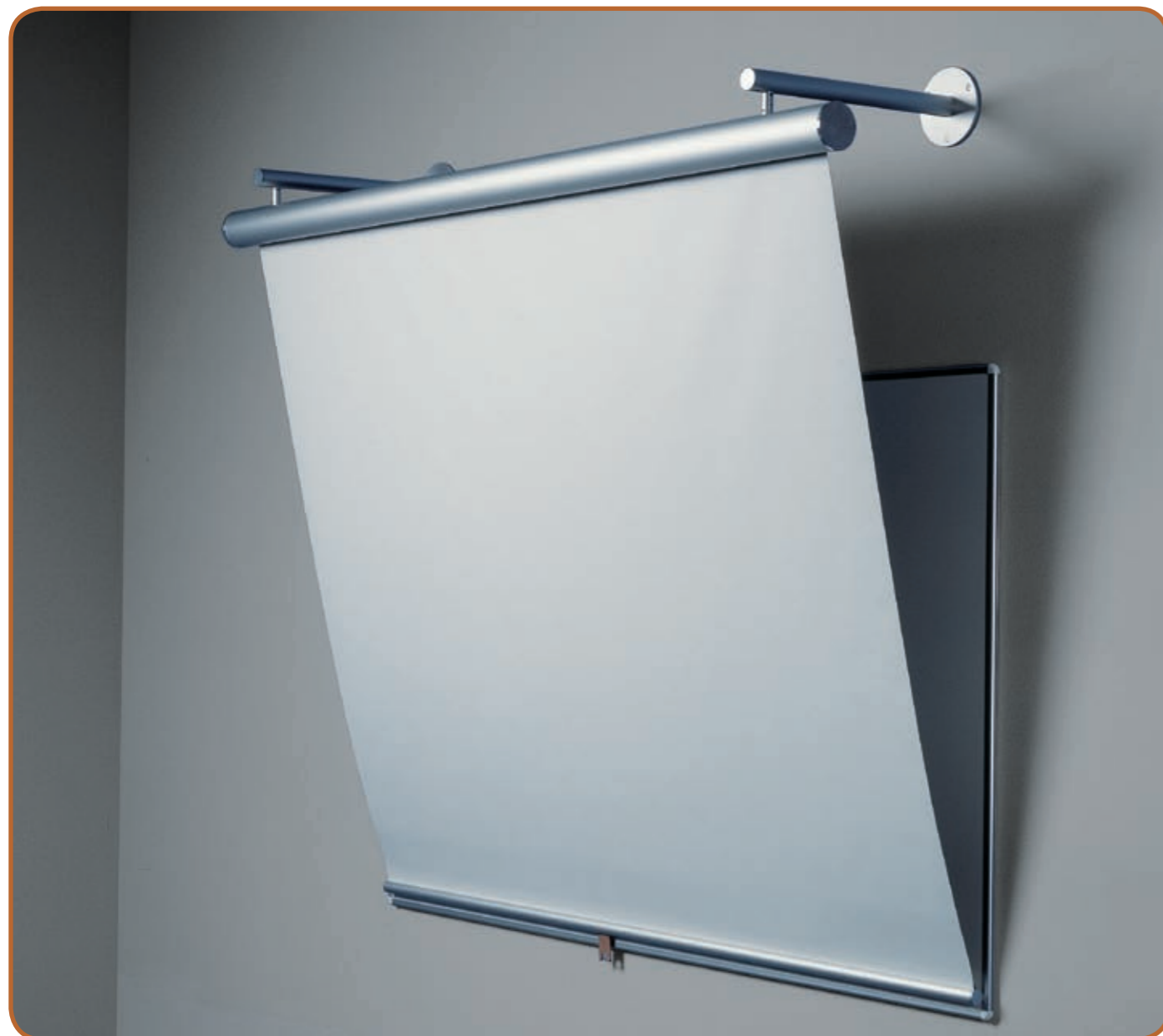
Silver Pipe Screen. Suitable for film, video, overhead or slide projection. Can be easily mounted on the ceiling or wall. The screen can either be tilted by fastening the strap to a wall hook or by using the small magnets in the bottom roller. Manually operated pull-down, crank handle operated or electrically operated screens. Gain figure approx. 1.0 up to a 50° visual angle.
